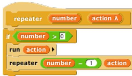
The lambda ( $\lambda$ ) next to **action** in the prototype indicates that this is a C-shaped block, and that the script enclosed by the C when the block is used is the input named **action** in the body of the script. The only way to make sense of the variable **action** is to understand that its value is a script.
